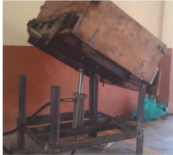
Fig.11. Prototype of tipper mechanism
